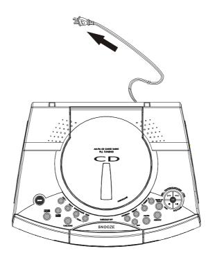
**<u>AM</u>**: The AM bar antenna is inside the cabinet of the main unit. You may need to change the position of the main unit until you find the position that provides the best reception for your favorite AM stations.
